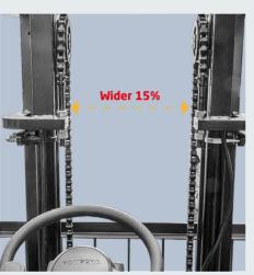
Adopt the new-type of box iron. Increase the inside width of inner mast and the spacing between lifting cylinders. The lowering of instruments in the driving cab will greatly increase the forward visibility; The rear visibility will also be greatly improved through the optimization design of counterweight.
