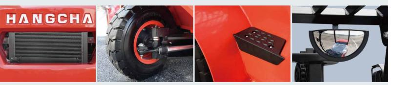
The radiator adopts aluminous plate-fin radiator with better performance and higher structural strength. Impendent oil radiator, optimized oil and water heat dissipation channel and double ventilation holes on counterweight can greatly improve cooling efficiency and reliability of overloaded operation and ensure reliable operation of the engine.
